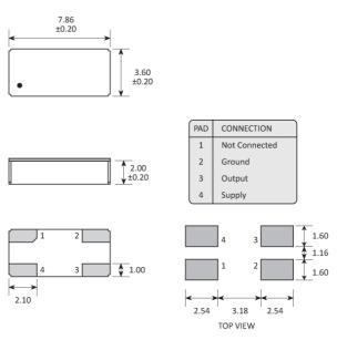
A 47nF ceramic capacitor must be connected between GND and VDD Dimensions in mm
