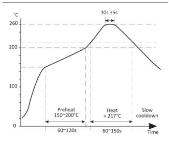
Lead free solderability limits:  $260^{\circ}C \pm 5^{\circ}C \times 10s \pm 5s \times 2$ .
