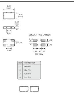
$\hbox{4-pole models consist of a match pair of units. They should be connected using the marks shown on each units.}\\$
