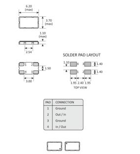
4-pole models consist of a match pair of units. They should be connected using the marks shown on each unit
