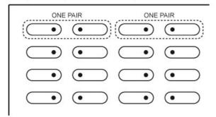
These filters are individually matched pairs. One filter is composed of two physical units, which have been factory-matched for optimum performance.
