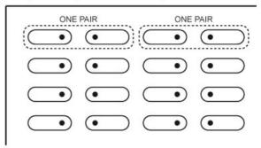
These filters are individually matched pairs. One filter is composed of two physical units, which have been factorymatched for optimum performance.
