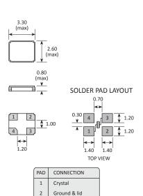
NOTE: Chamfer normally on pad 4, but may alternatively be supplied on pad 1.
