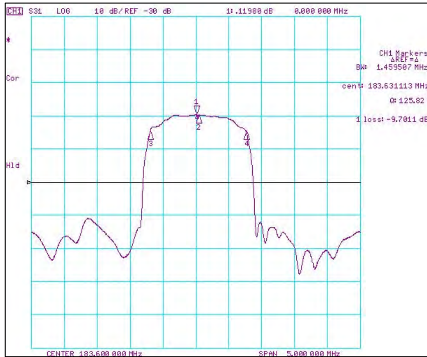
Fig-1 S21 Response Horizontal: 0.5MHz/Div Vertical: 10dB/Div. Reference: -30dB
