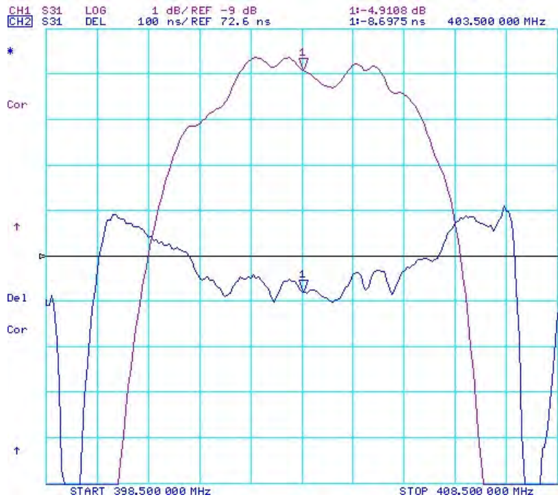
Group Delay and Ripple, Horizontal:1 MHz/Div Vertical 1: 1 dB/Div Vertical 2: 100 nS/Div
