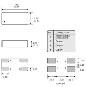
A 47nF ceramic capacitor must be connected between GND and  $\mathsf{V}\mathsf{D}\mathsf{D}$
