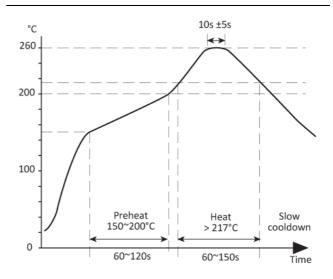
Lead free solderability limits:  $260^{\circ}C \pm 5^{\circ}C \times 10s \pm 5s \times 2$ .
